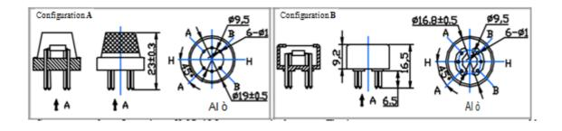
Structure and configuration of MQ-135 gas sensor is shown as Fig. 1 (ConfigurationA or B), sensor composed by micro AL2O3 ceramic tube, Tin Dioxide (SnO2) sensitive layer, measuring electrode and heater are fixed into a crust made by plastic and stainless steel net. The heater provides necessary work conditions for work of sensitive component
