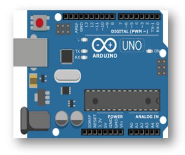
The Arduino Uno is an open-source microcontroller board based on
