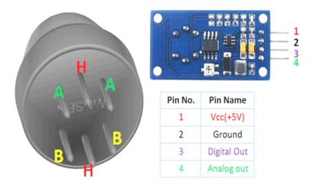
MQ-135 Gas Sensor Pin out
