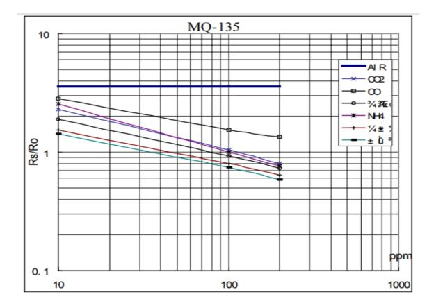
The above figure shows the typical sensitivity characteristics of the MQ-135 for several gases in their: Temp: 20, Humidity: 65%, O2concentration21%,  $RL=20k\Omega$ ,
