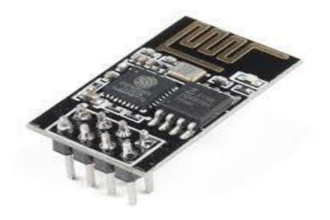
The ESP32 WiFi Module is a self contained SOC with integrated TCP/IP protocol stack that can give any microcontroller access to your WiFi network. The ESP8266 is capable of either hosting an application or offloading all Wi-Fi networking functions from another application processor.
