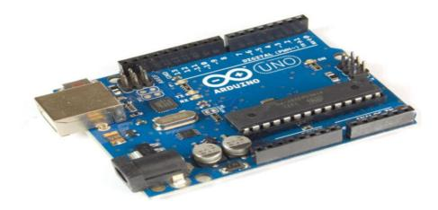
The Arduino Uno is a microcontroller board based on the ATmega328 (datasheet). It has 14 digital input/output pins (of which 6 can be used as PWM outputs), 6 analog inputs, a 16 MHz crystal oscillator, a USB connection, a power jack, an ICSP header, and a reset button. It
