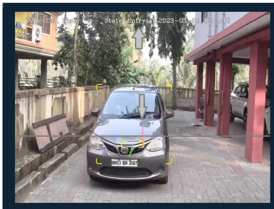
Image showing the gate line for detection (gray horizontal line) with green arrow indicating vehicle movement direction, and red arrow indicating direction of gate normal.
