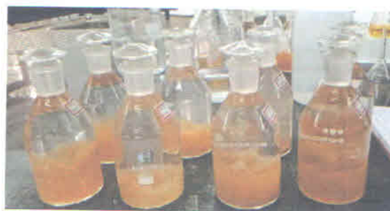
Fig 7. D.O bottles after fixing with Winkler's A and B
