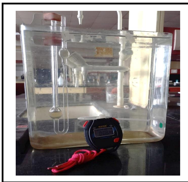
Figure 4: Borosil viscometer used to measure viscosity
