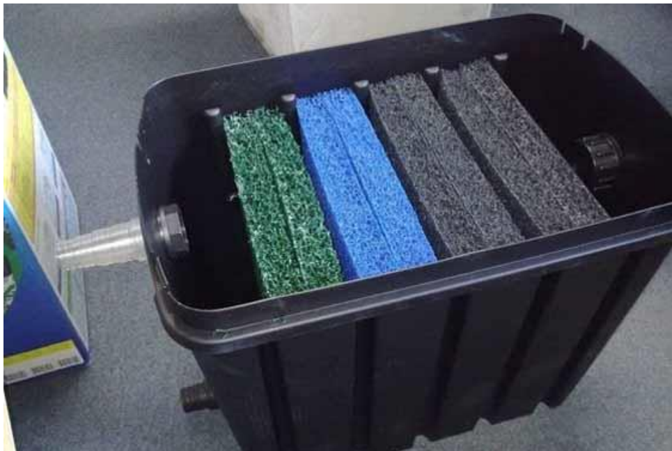
Figure.18. Mechanical filter unit
