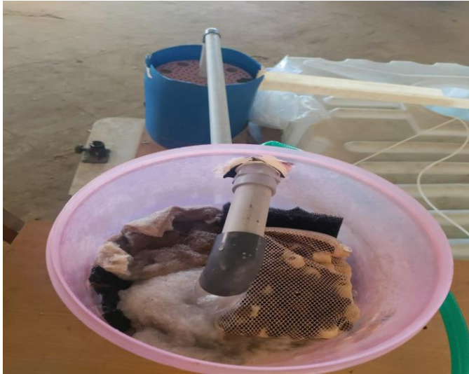
Figure.22. water flowing from tank to bio filter via mechanical filter.
