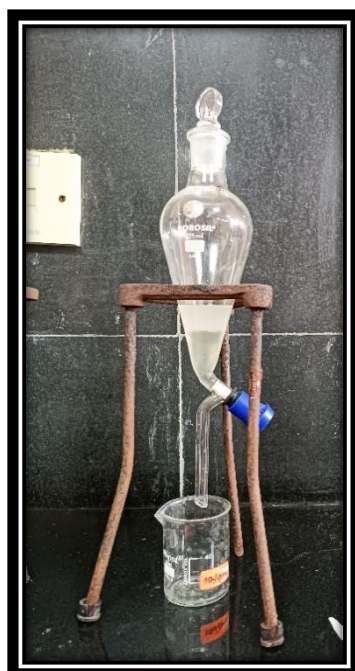
Plate 5: Phase separation in fatty acid test
