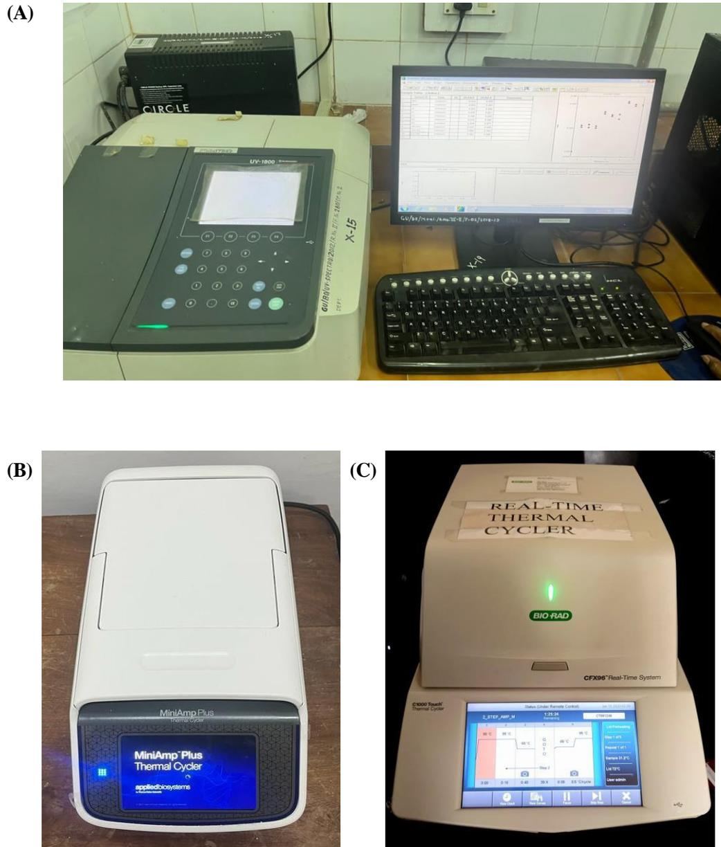
**Figure 3.2.** Instruments operated to carry out experiments under study (A) UV Visible spectrophotometer (UV 2450, Shimadzu), (B) Thermocycler (MiniAmp™Plus Thermal cycler), (C) BioRad Real-Time PCR
