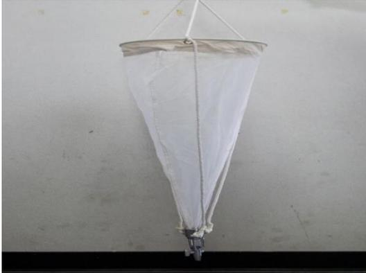
Figure 7: Phytoplankton net (“A simple plankton met with 20-micron mesh size.jpg” by Warichrb29 is licensed under CC SA 4.0)
