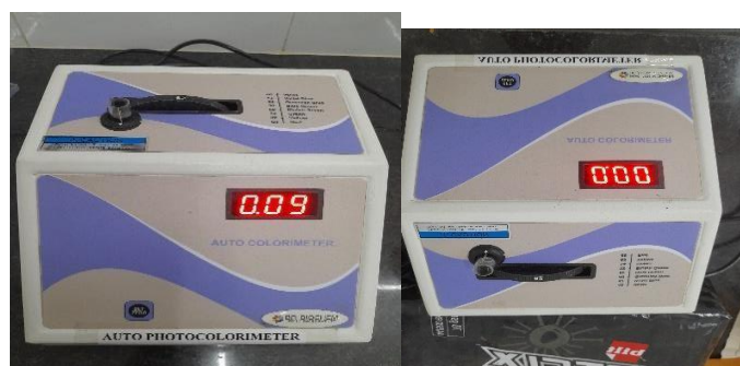
Fig 7: Auto Photo colorimeter used to differentiate between archaea and bacteria.
