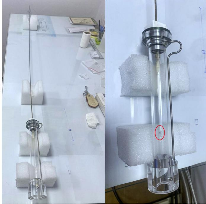
Figure 2.10: Sample inserted into the sample rod
