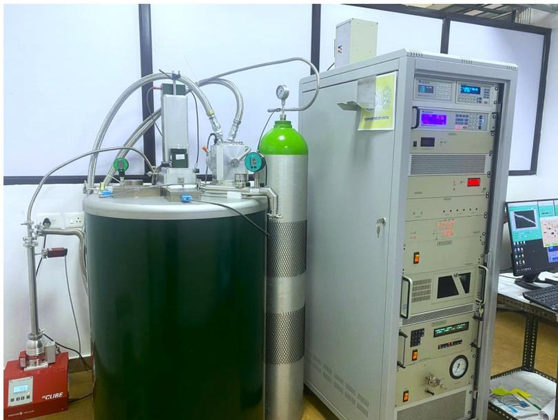
Figure 2.9: Cryogenic Laboratory SQUID Magnetometer at MCL, Goa University
