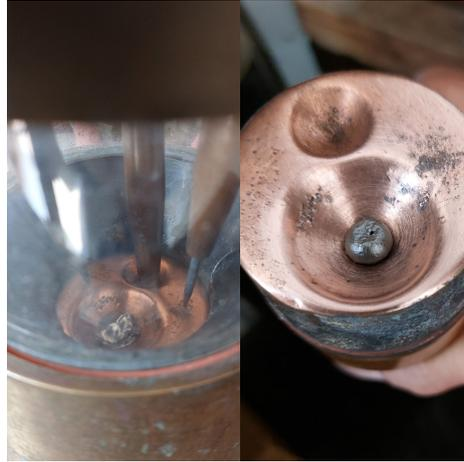
Figure 2.4: Samples in Arc Furnace
