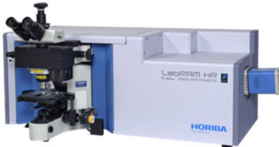
Figure 4.11 LabRAM HR Evolution Raman Microscope
