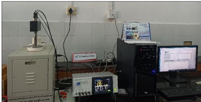
Figure 3.16 Electrical Network Analyser
