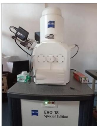
Figure 4.5 Carl Zeiss Scanning Electron Microscope Setup
