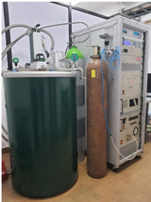
Figure 4.8 SQUID magnetometer
