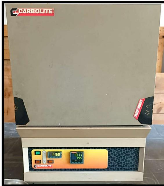
Figure 2. 1 Furnace used for melting of batch of glass.
