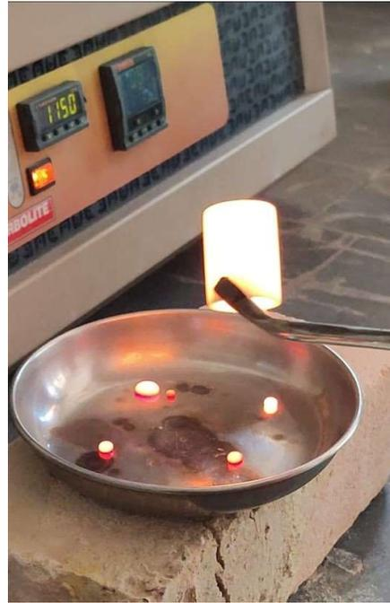
Figure 3. 3 Droplets of glass Formation of Glass
