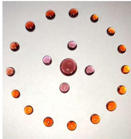
Figure 3. 5 Photo of glass  $\text{H}_3\text{BO}_3\text{-Bi}_2\text{O}_3\text{-SrCO}_3\text{-Nd}_2\text{O}_3$  with varying composition of Neodymium
