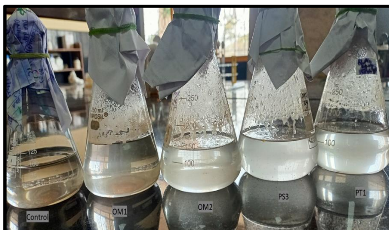
Fig 3: Growth of individual isolates in BHB with 1% Oil as carbon source after 7 days of enrichment
