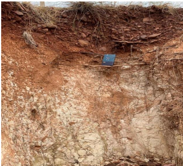
Fig 6: cross section of A thick layer of conglomerate, 20cm notebook as a reference.
