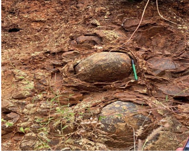
Fig 4. Spheroidal weathering of basalt, a pen as a reference.
