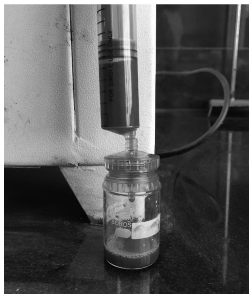
Fig 13: Filtered digested clams solution passed through 0.22 \mu m Whatman filter using a 20mL syringe
