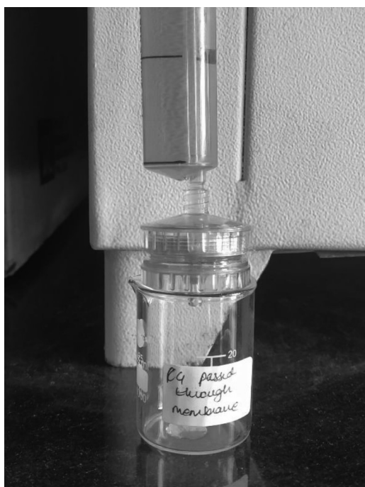
Fig 12: Filtered digested chicken gut solution passed through 0.22 \mu m Whatman filter using a 20mL syringe
