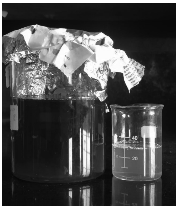
Fig 6: Digested solution treated with 100% EtOH
