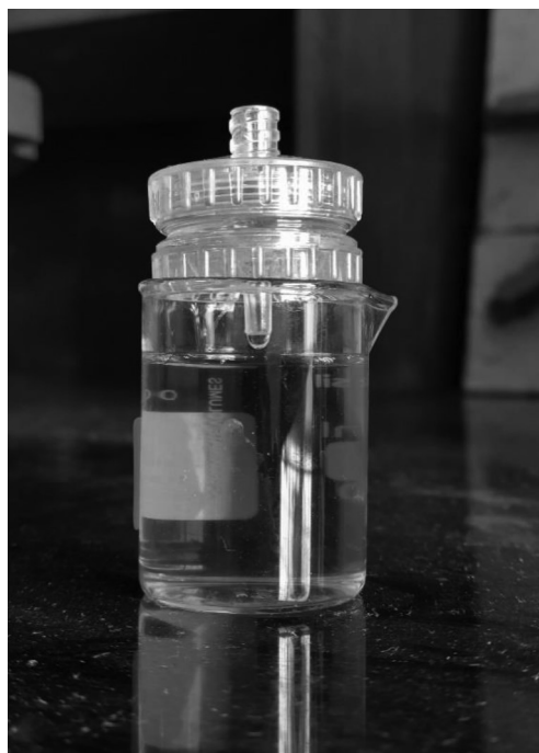
Fig 12: Filtered digested chicken gut solution passed through 0.22 \mu m Whatman filter using a 20mL syringe
