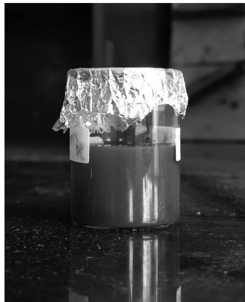
Fig 13: Filtered digested clams solution passed through 0.22 \mu m Whatman filter using a 20mL syringe
