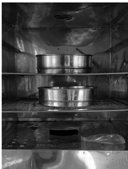
Fig 10: Sieves kept in hot air oven at 60°C
