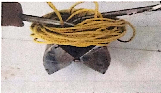
Fig 5: Van Veen Grab (for sediment collection)
