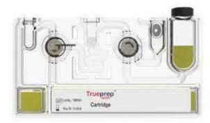
Disposable plastic cartridge for automated extraction of nucleic acids from clinical specimens.
