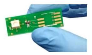
Disease specific, ready-to-use and disposable micro-PCR chips that run on the Truelab Uno Dx/ Duo/Quattro to get quantitative real time PCR results.
