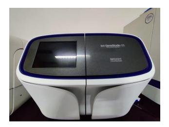
The **Ion GeneStudio S5 System** is a semiconductor-based nextgeneration sequencing (NGS) system that enables simple targeted sequencing workflows. The Ion GeneStudio S5 System is optimized to provide affordability for labs focused on smaller panels and lower sequencing throughput requirements.
