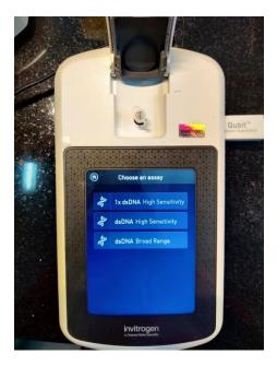
Qubit Fluorometers detect fluorescent dyes specifically bound to the target molecule. With optimized Qubit Assays, they can distinguish dsDNA from ssDNA or intact from degraded RNA, even in extremely small amounts or in the presence of contaminants. A simple, intuitive interface and onboard calculators streamline the process. Results appear within seconds and can be exported to a computer or downstream device.
