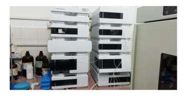
HPLC is a separation technique in which liquid is used to force the sample at high pressure through a column packed with stationary phase in order to identify and/or quantify the components.
