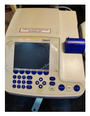
The **Eppendorf BioSpectrometers** are small, very compact spectrophotometers that allow users to conduct measurements in the UV/ Vis and fluorescence range. Absorbance spectra can be recorded, and individual wavelength measurements can be conducted, in a spectral range of 200 nm to 830 nm.
