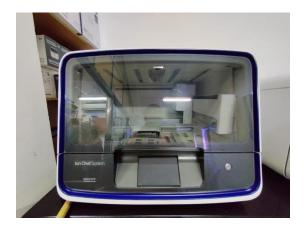
The **Ion Chef System** provides automated library preparation, template preparation, and chip loading for users. In less than 15 minutes of upfront hands-on time and with the use of pre-packaged library preparation reagent kits, the Ion Chef System provides a convenient walk-away workflow resulting in equalized, pooled libraries ready for templating. The automated workflow supports Ion AmpliSeq one- and two-pool designs.
