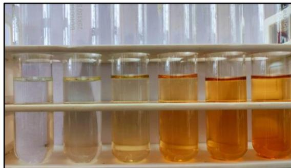
Fig. 53. Test tubes depicting a series of standards of Ammonia prepared with Ammonium chloride.
