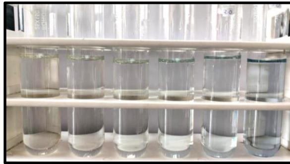
Fig. 7. Test tubes depicting a series of standards of phosphates prepared with potassium dihydrogen orthophosphate.
