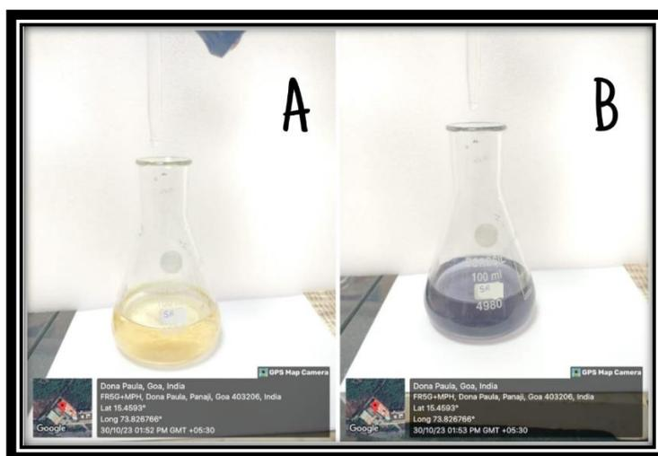
Figure 5: Titrating of DO sample against  $\text{Na}_2\text{S}_2\text{O}_3$  A : Before addition of starch indicator. B:
