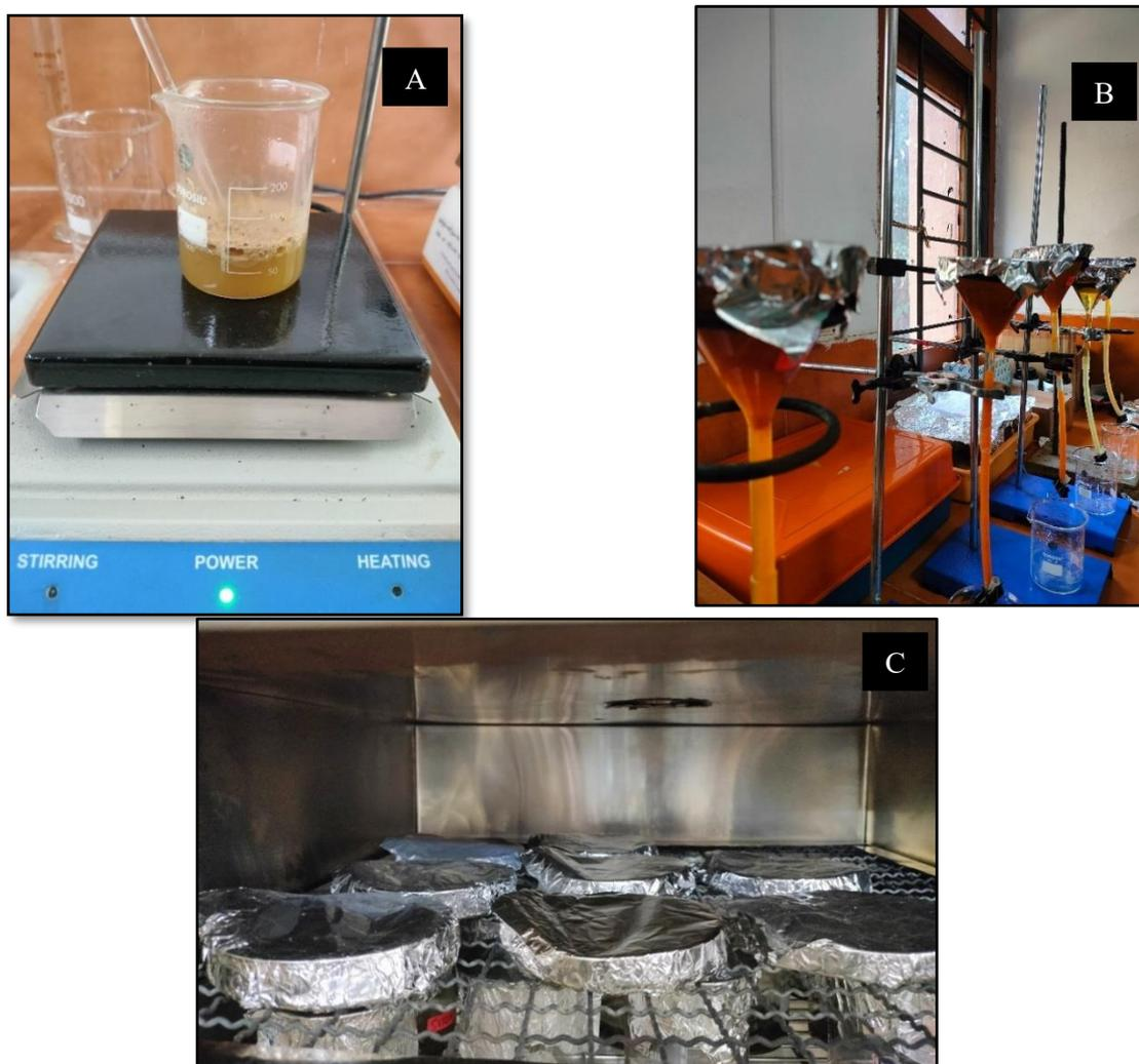
Figure 3.8: Laboratory Analysis, (A; dissolving organic matter, B; density separation setup, & C oven drying of petri dishes
