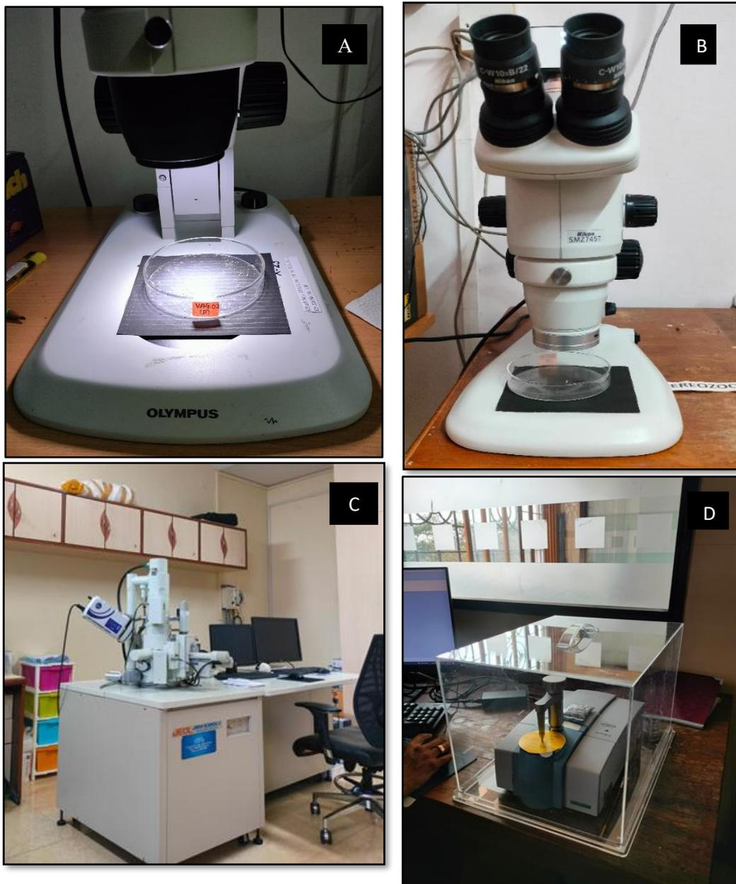
Figure 3.9: Instruments Used in Microscope Examination. (A & B; Stereozoom Microscope, C; Scanning Electron Microscope, D; Interferometer).
