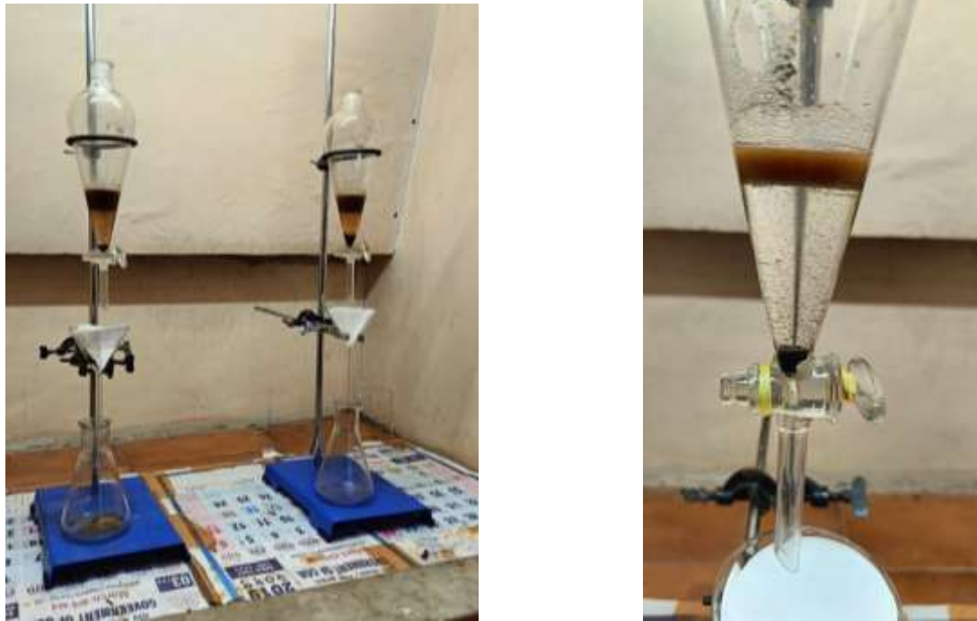
Figure 3.8 Bromoform Analysis settled heavy minerals and floating light minerals.
