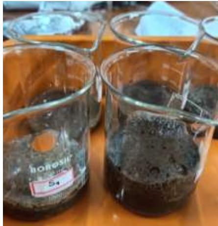
Figure 3.5 Vigorous reaction after H 2 O 2 treatment
