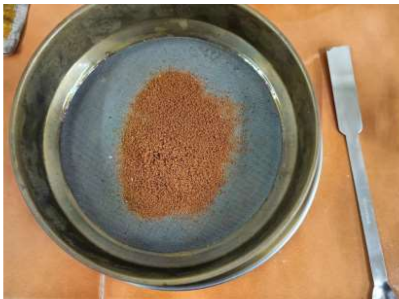
Figure 3.7 Separated fine grain <400\mu\text{m}
