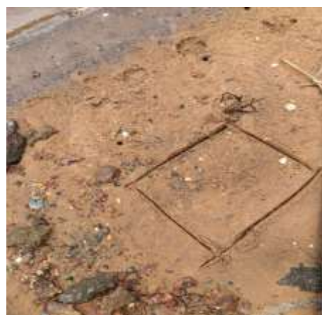
Figure 3.3 15cmx15cm square for a good representative sample
