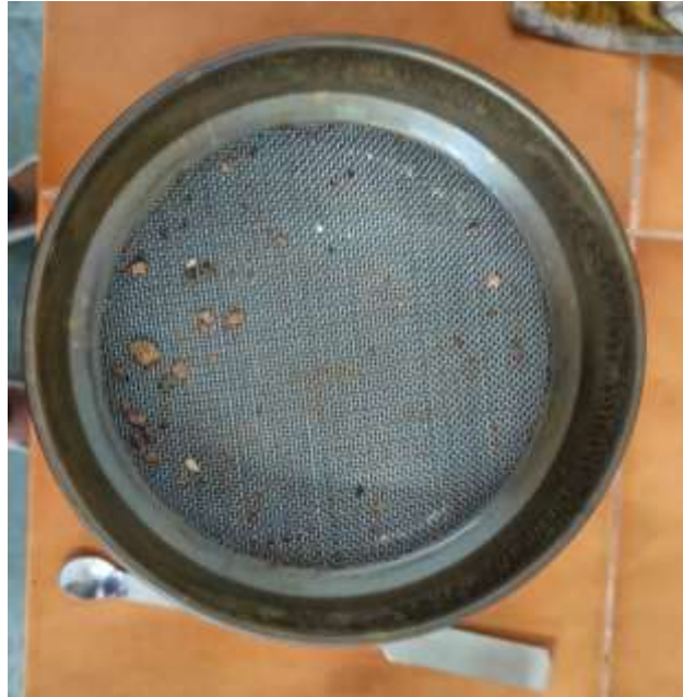
Figure 3.6 Separated coarse grain >400\mu\text{m}
