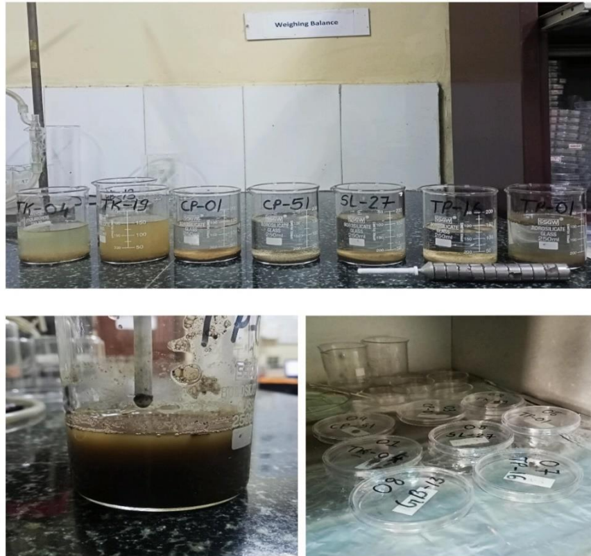
figure 13: sample processing for magnetic mineral separation
