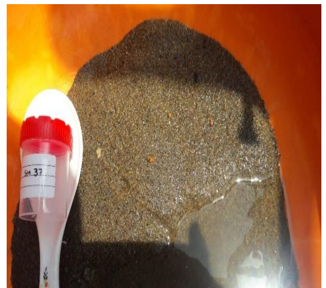
Fig 7: Bulk Sediment collection from grab sampler and collected bulk sediment samples.
