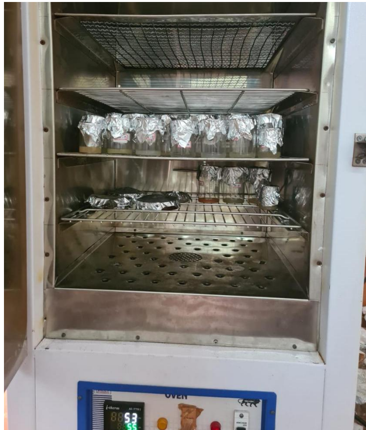
Figure 3.11: Sand fraction collected from the sieves kept for drying in oven
