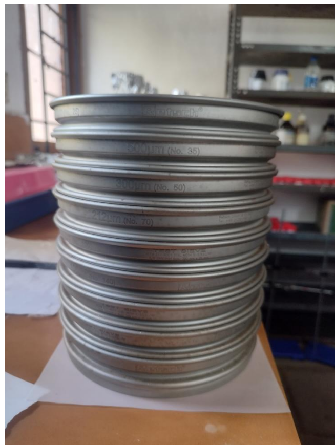
Figure 3.10 : Sieves used for sieving sand fraction
