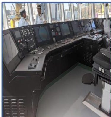
Integrated Platform Management System
