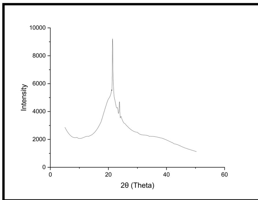
**Fig.4.11. X-ray diffraction profile of selenium nanoparticles synthesized from ASB12**
