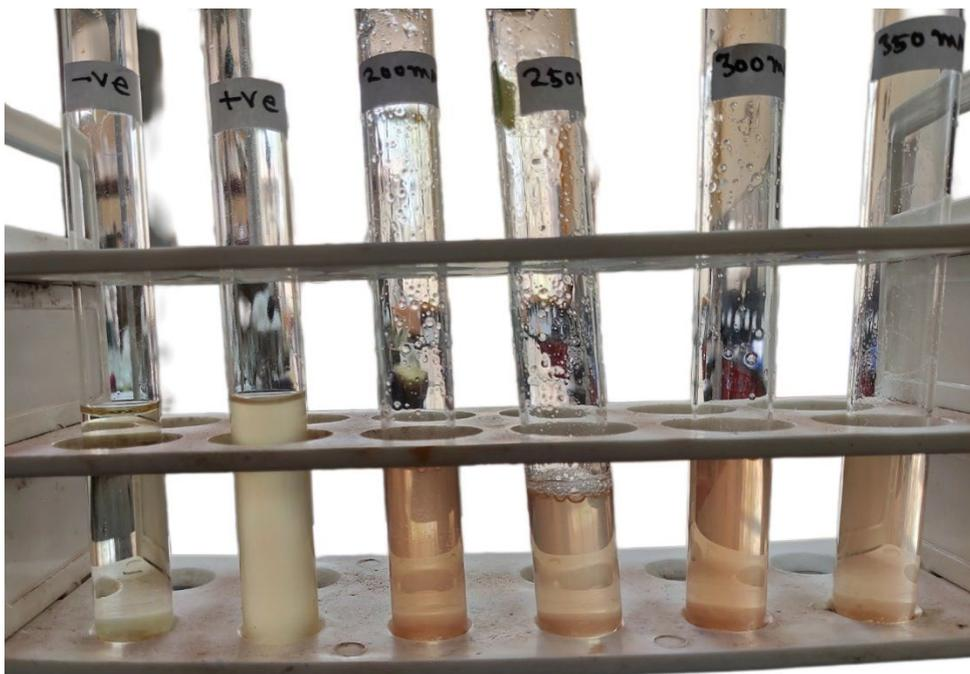
**Fig.4.5. Tubes containing sodium selenite concentrations of 200 mM, 250mM, 300 mM and 350 mM showing effect on growth of ASB12**
