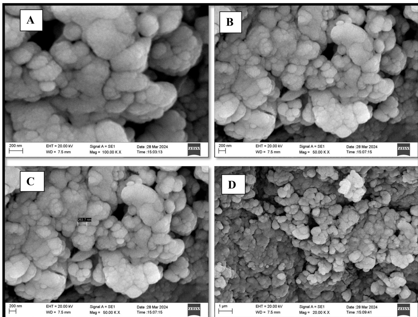
**Fig. 4.12. SEM micrographs of selenium nanoparticles synthesized from ASB12**
