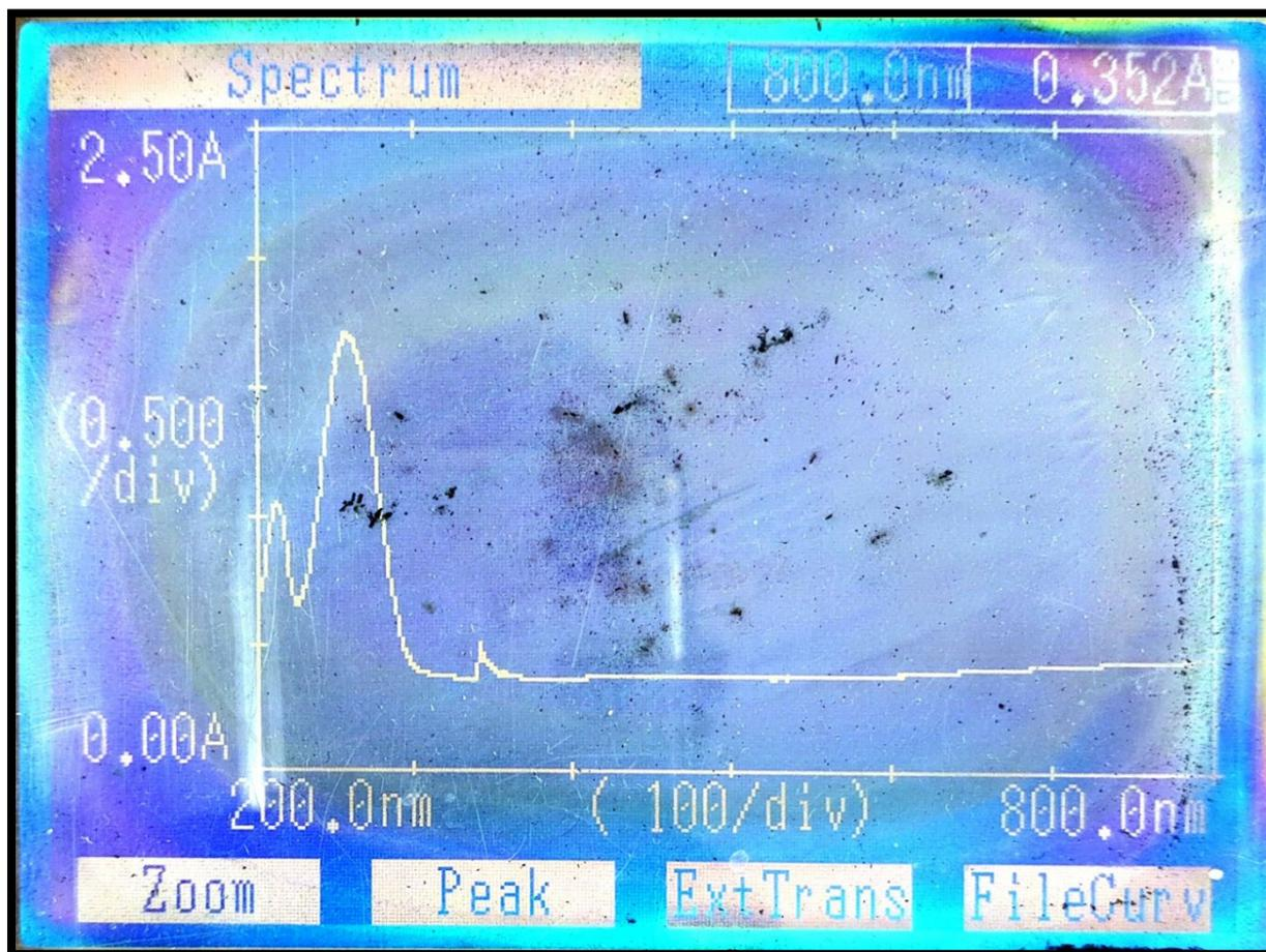
Fig. 4.8. UV-vis spectrum of selenium nanoparticles synthesized from ASB12
