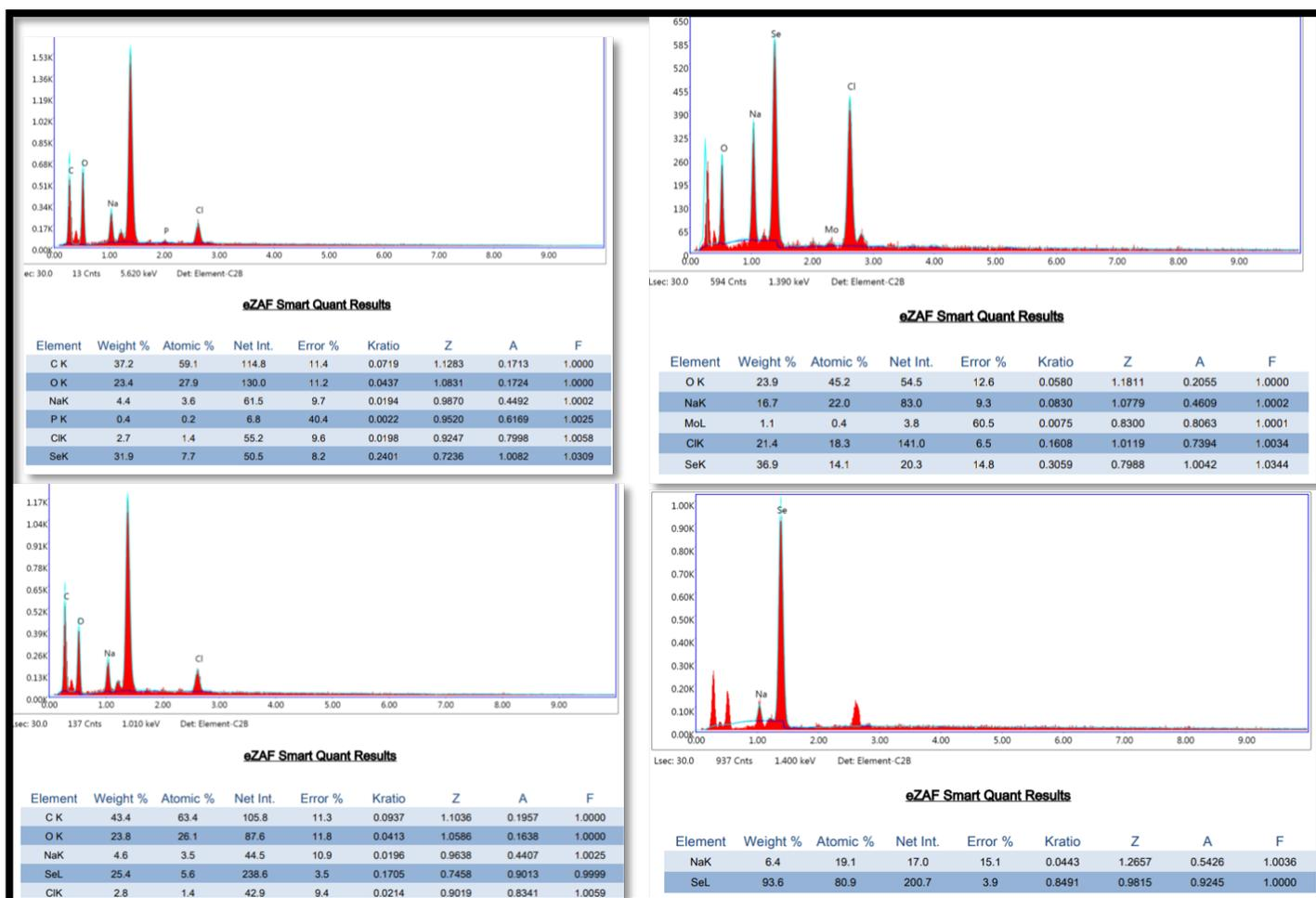
**Fig. 4.14.** EDX profile image of selenium nanoparticles synthesized from ASB12
