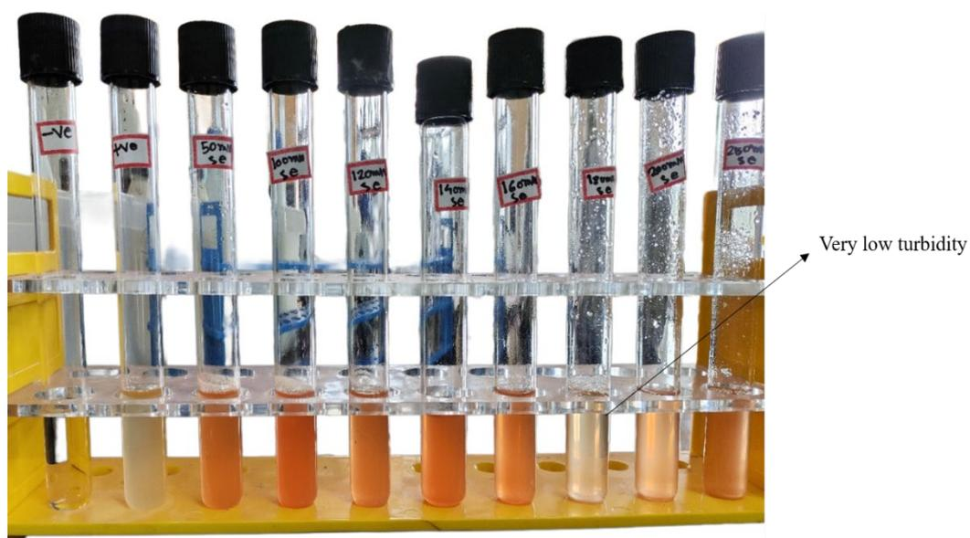
Fig.4.4. Tubes containing sodium selenite concentrations up to 250 mM showing effect on growth of ASB12
