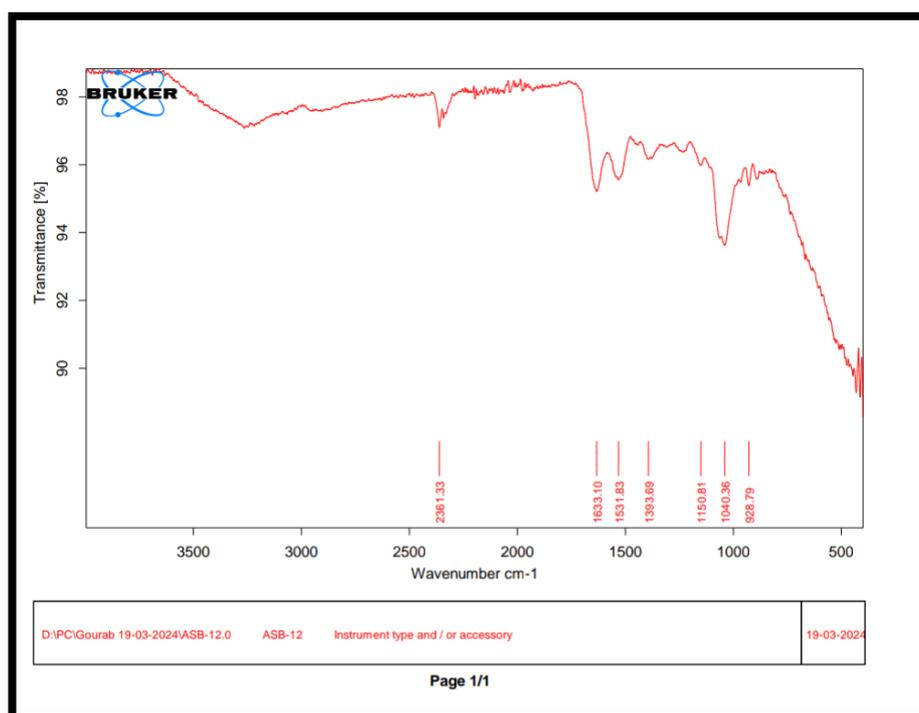
**Fig.4.13. Fourier-transform infrared spectrum of powdered selenium nanoparticles synthesized from ASB12**
