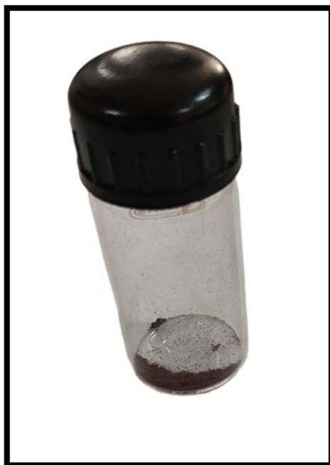
**Fig. 4.9. Powdered Selenium nanoparticles in glass vial**
