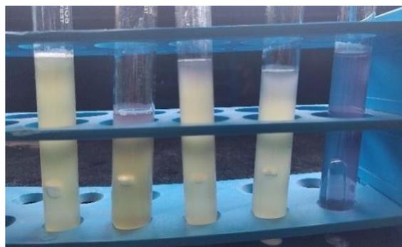
Fig 3.4: MPN 1x tube shows test tubes 1 to 4 giving positive results and tube 5 shows negative results
