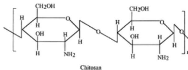
Figure 1.4: Structure of Chitosan (Dave et al., 2021)
