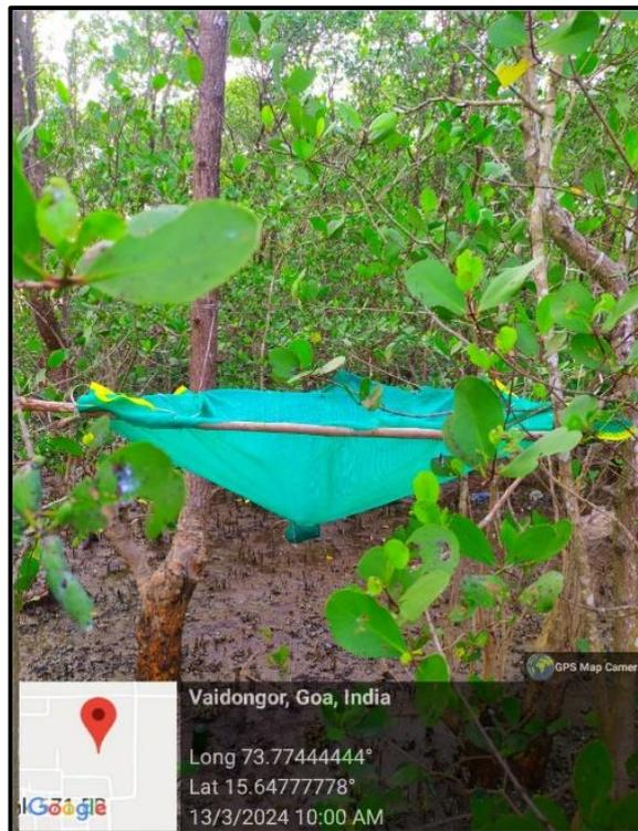
**Fig. 3.3.** Litter trap installed at VD-3 at the mid tide zone.
