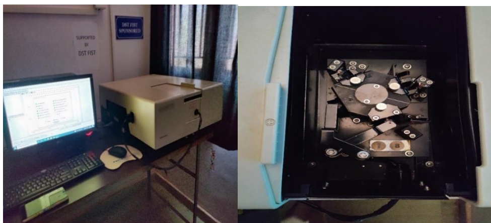
Figure 23 UV-Vis spectroscopy setup for powder sample
