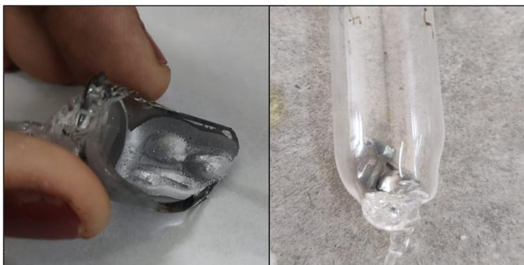
Figure 3.6: Sn melted out of the sample on annealing
