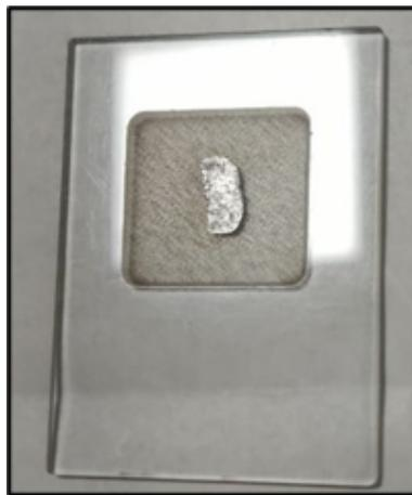
Figure 3.1: Sample pounded into a thin sheet
