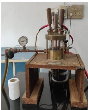
Figure 2.1: Arc Furnace
