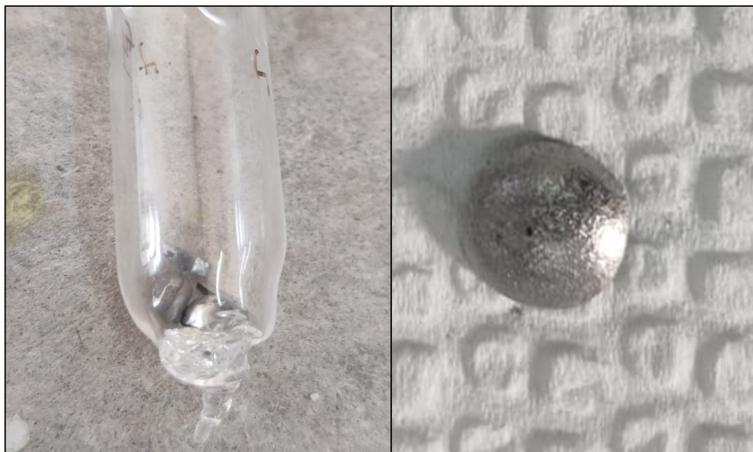
Figure 3.11: Sample fused together on annealing
