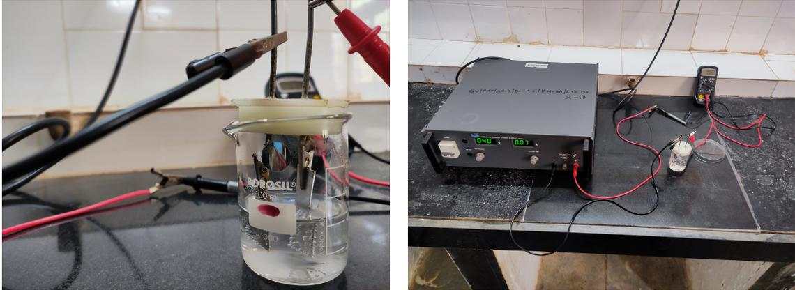
Figure 3.1: Electrode setup of Anodization of Aluminum (left) and Anodization process complete setup (right)
