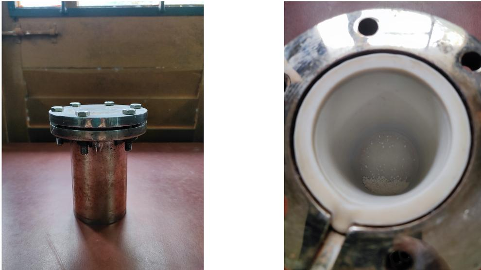
Figure 3.2: Hydrothermal Autoclave image (left) & Teflon beaker fitted in autoclave (right)
