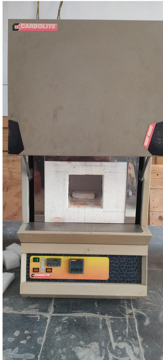
Figure 2.3: Furnace for annealing sample
