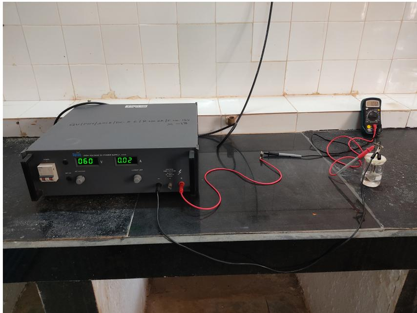
Figure 1.2: Anodization setup
