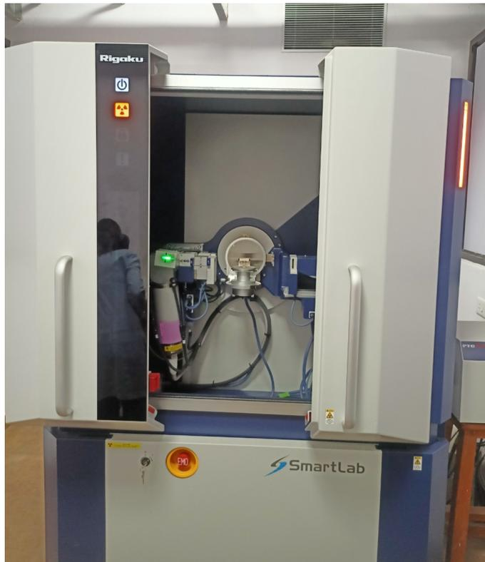
Figure 6: X-ray diffractometer (XRD)
