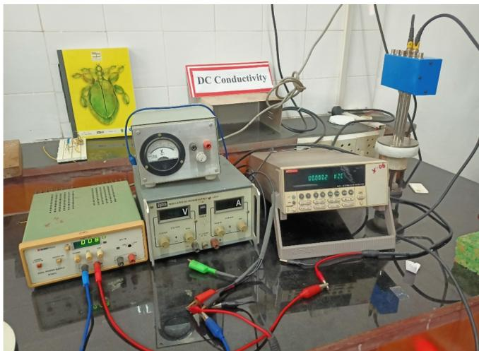
Figure 12: Dc conductivity setup
