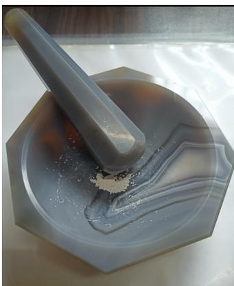
Figure 5: Mortar and pastle used for grinding
