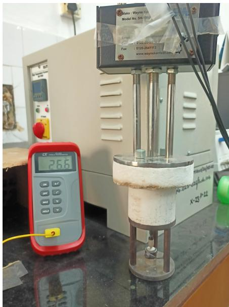
Figure 15: Measurement of impedance data of sintered pellet
