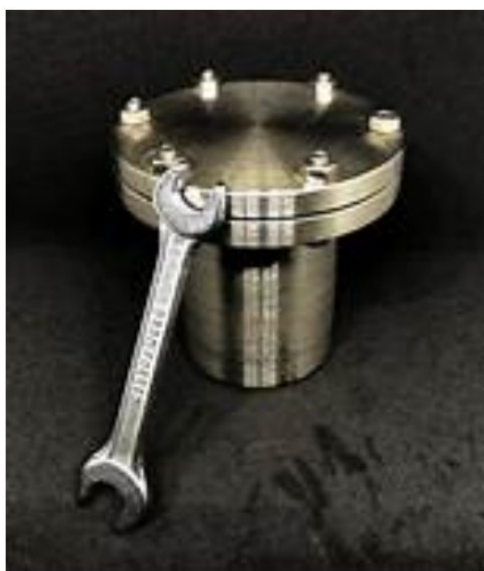
Figure 2: Autoclave used in hydrothermal method (SPAS Goa University)
