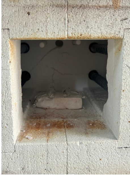
Figure 2.5: quartz ampoule in furnace
