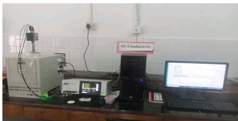
Figure 21: Experiment set-up of electrochemical impedance spectroscopy technique (EIS)
