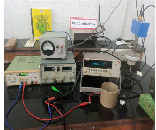
(b) Experiment set-up of DC polarization technique
