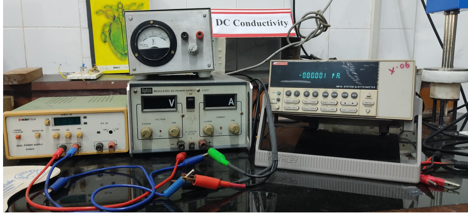
Figure 3.9: DC Conductivity setup
