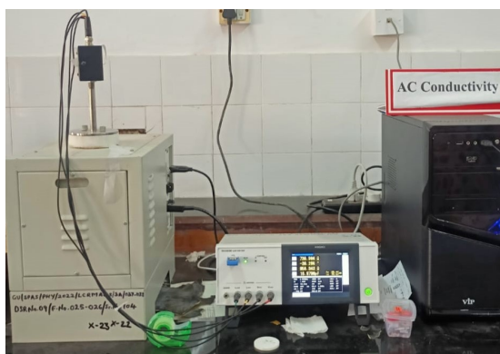
Figure 3.4: AC Conductivity setup
