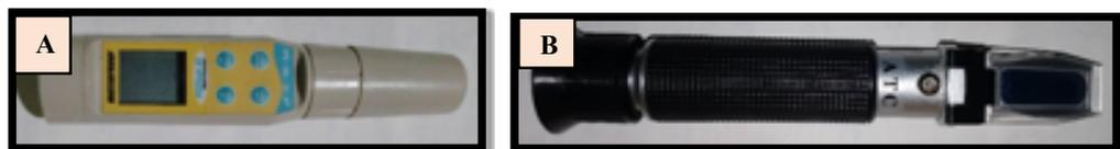
Fig 3.5 A. depicting PCS testr 35 and B. hand held refractometer used for maintaining water quality parameters and salinity in ppt respectively.
