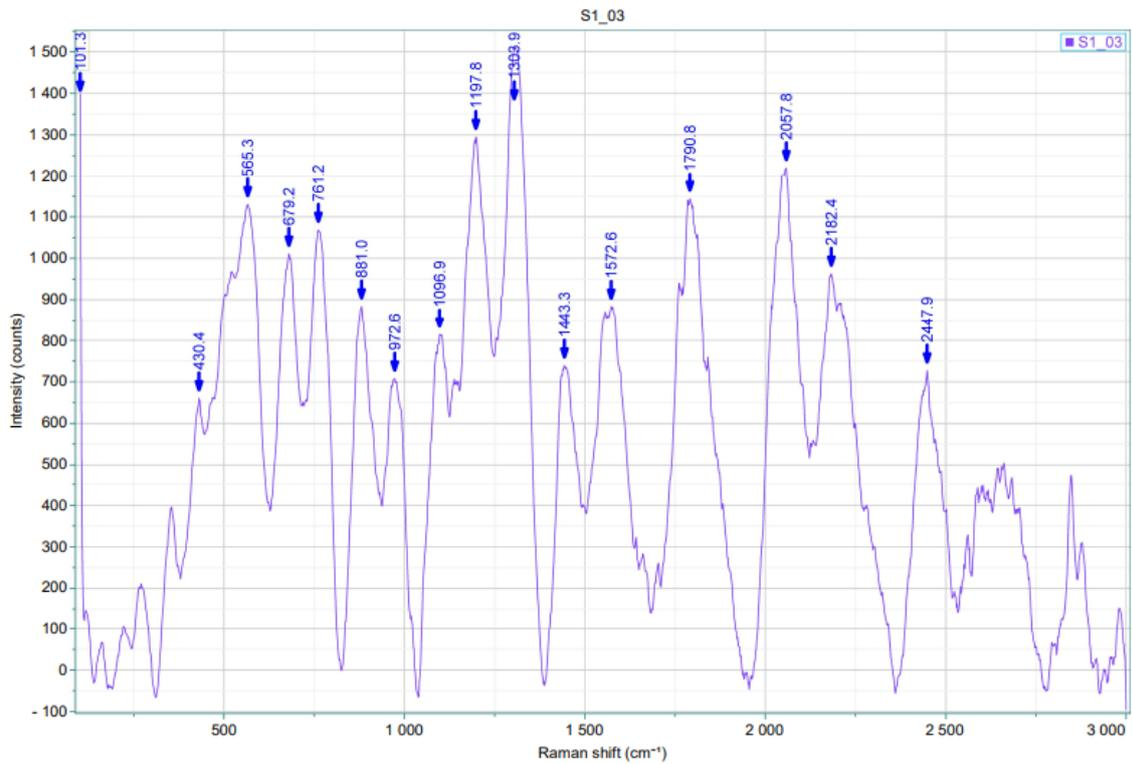
Fig 8 :- Raman Spectra of unknown microplastic identified as a Polyethylene Terephthalate
