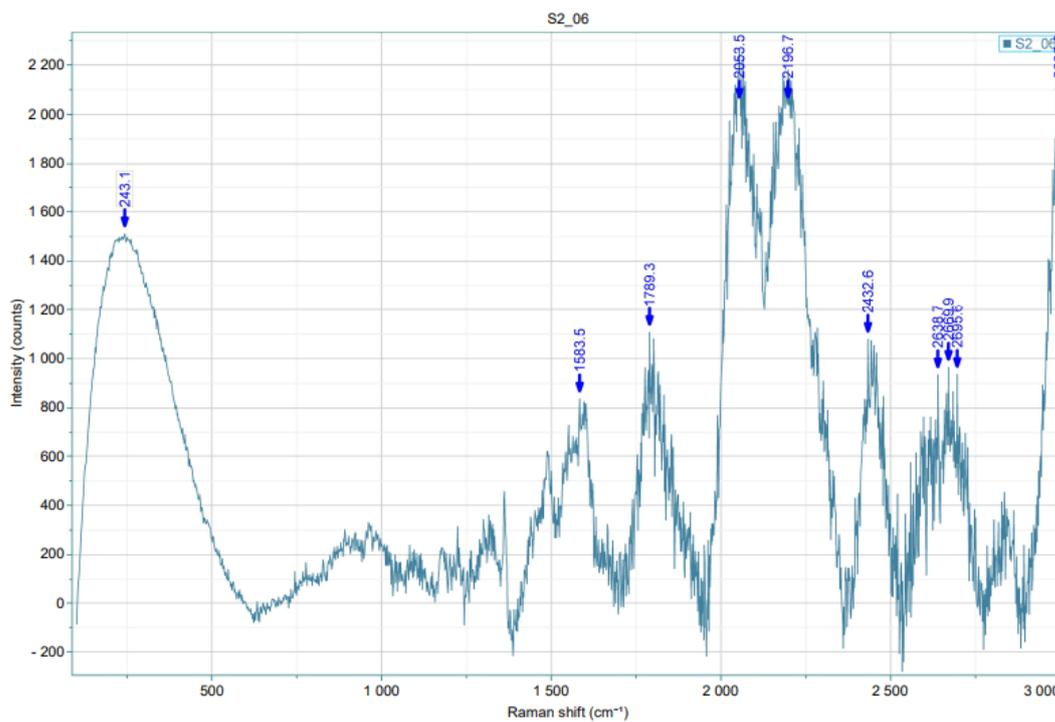
Fig 4 :- Raman Spectra of unknown microplastic identified as a Polyacrylonitrile
