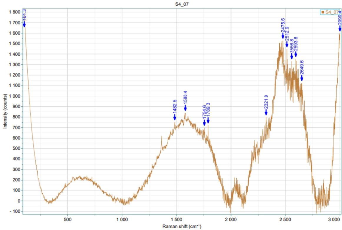
Fig 6 :- Raman Spectra of unknown microplastic identified as a Epoxy
