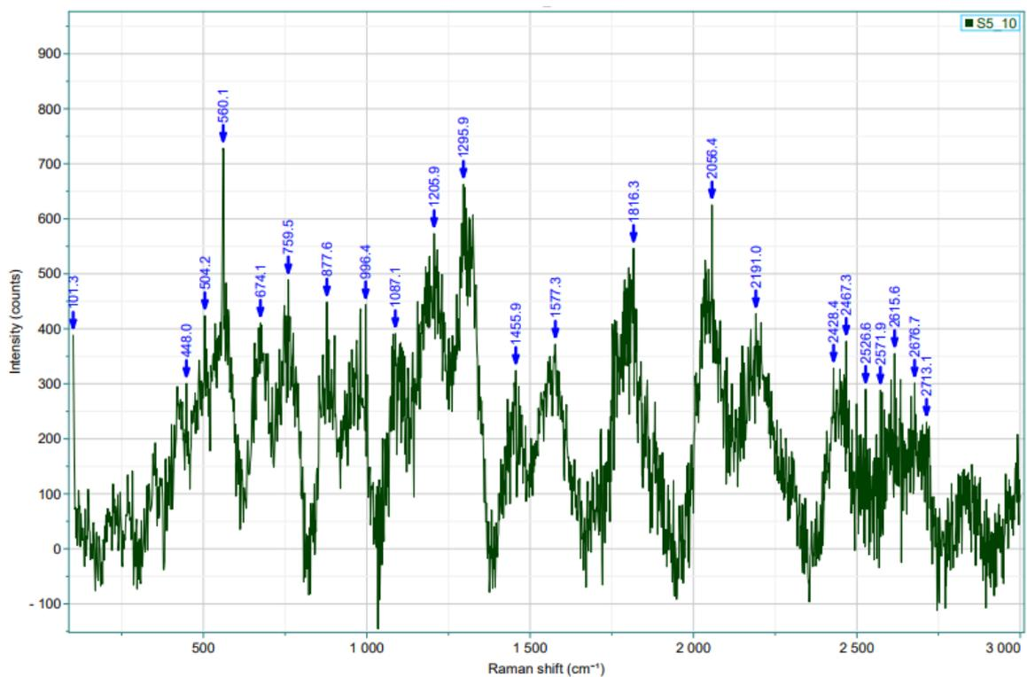
Fig 7 :- Raman Spectra of unknown microplastic identified as a Polyvinyl Chloride
