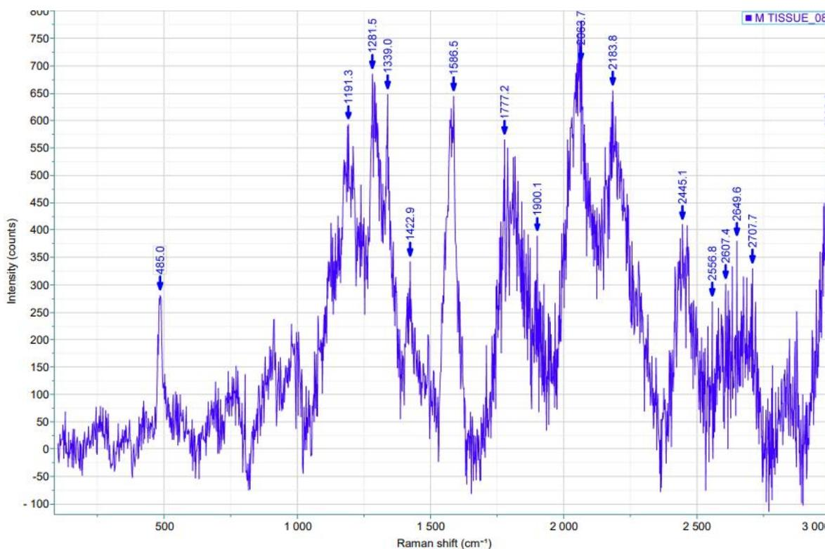
Fig 5 :- Raman Spectra of unknown microplastic identified as a Polyamide
