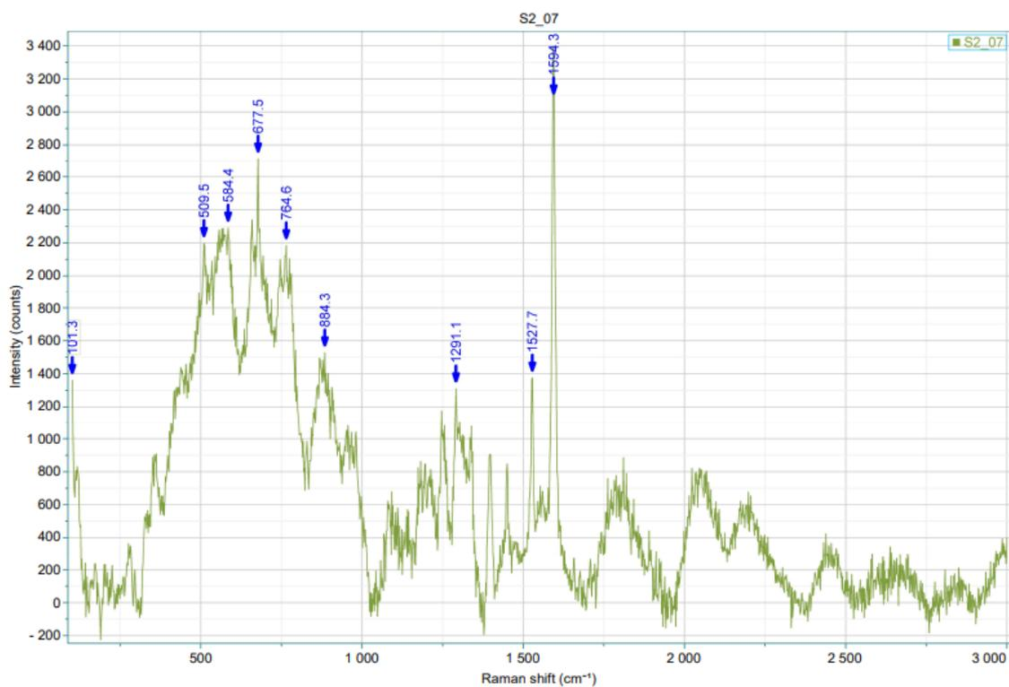
Fig 3 :- Raman Spectra of unknown microplastic identified as a Polycarbonate
