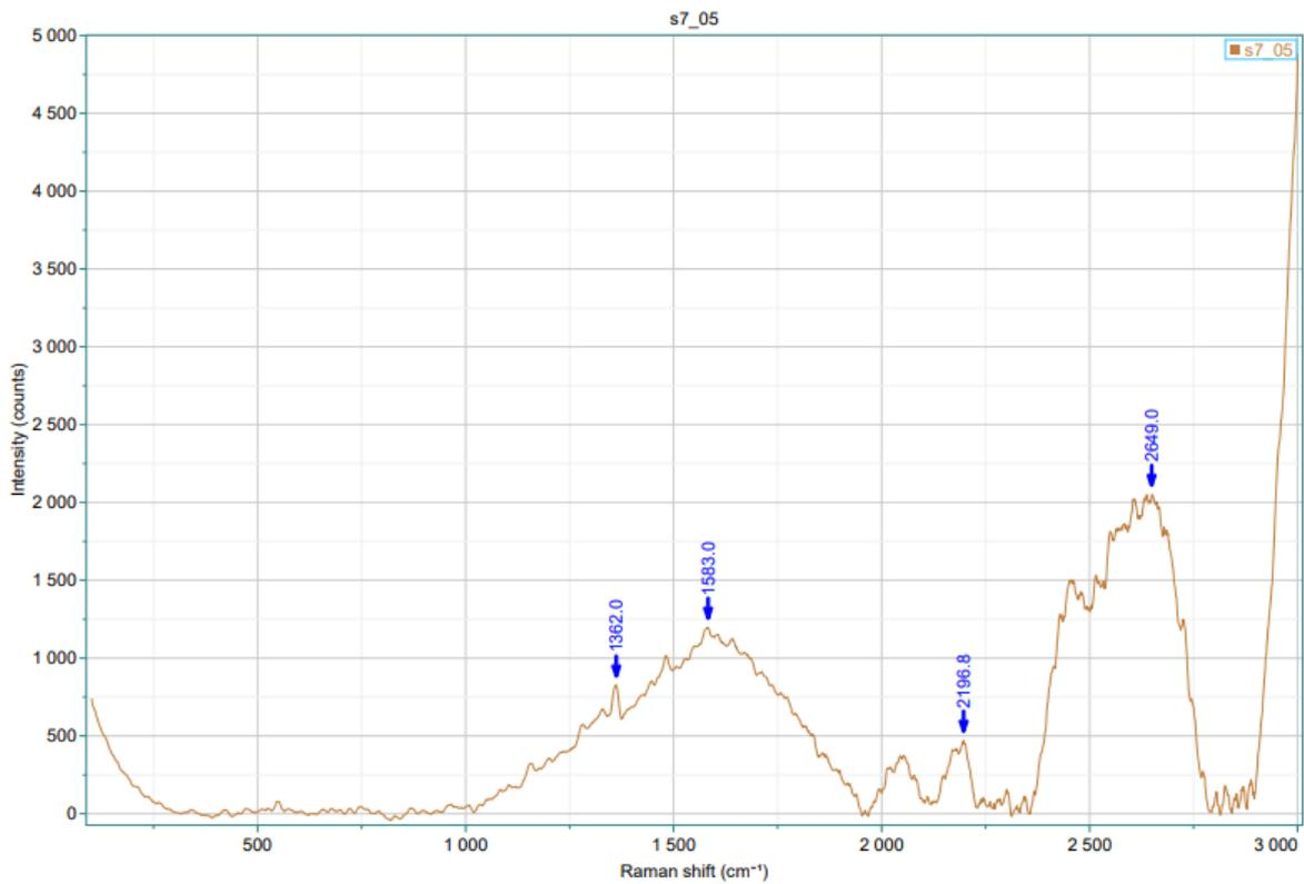
Fig 9 :- Raman Spectra of unknown microplastic identified as a Polyethylene Vinyl acetate
