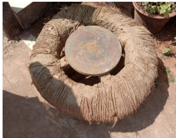
Fig. 3.4 Potter's wheel tied with jute rope and mud paste, Mastimol, Canacona
