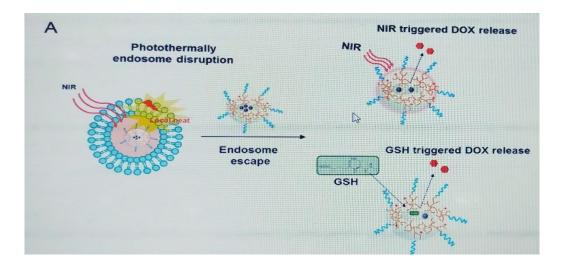
Fig B:Photothermal disruption of endosome to release DOX drug in cytoplasm
