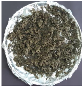
The sample dried at room temperature, placed in the oven at 60°C for 5 h
