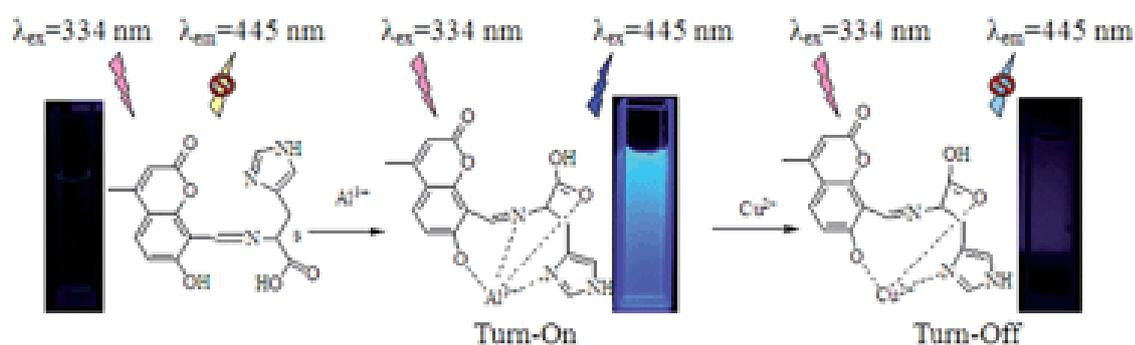
Fig. 6 mechanism of the chemosensor for the detection of  $\text{Al}^{3+}$ .
