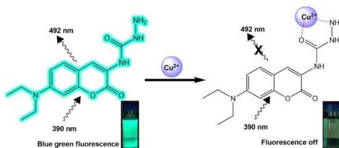
Fig.2 sensing mechanism of  $\text{Cu}^{2+}$  ions by chemosensor.
