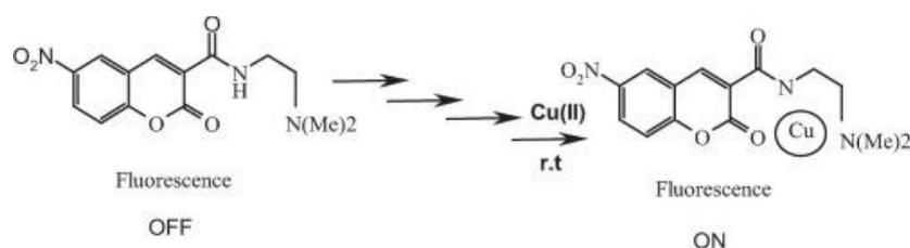
Fig. 8 chemosensor for detection of Cu<sup>2+</sup>.
