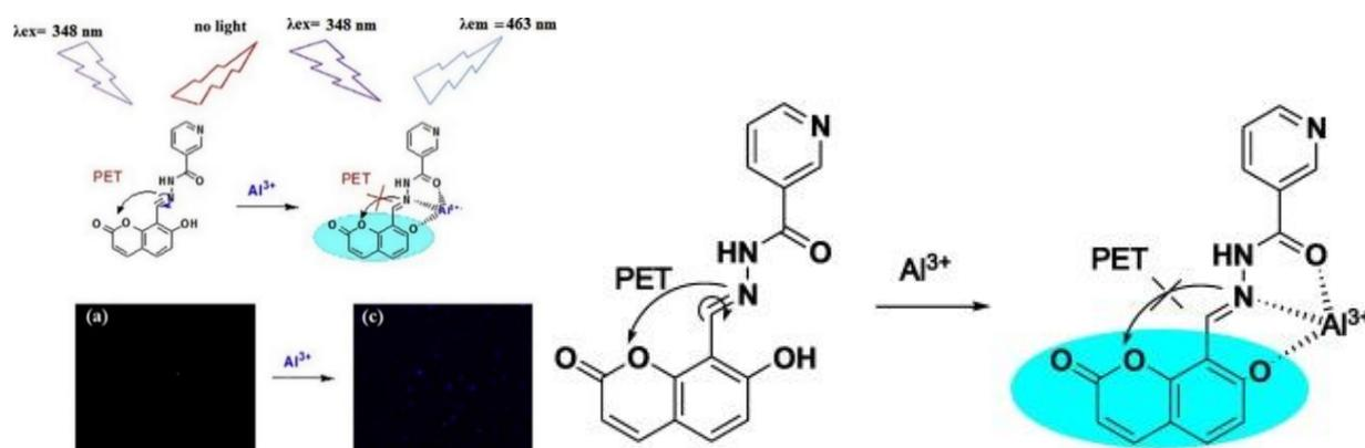
Fig.3 Mechanism of the sensor for detection of  $\text{Al}^{3+}$ .
