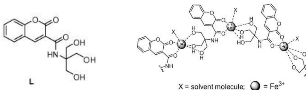
Fig. 5 chemosensor for detection of  $\text{Fe}^{3+}$ .
