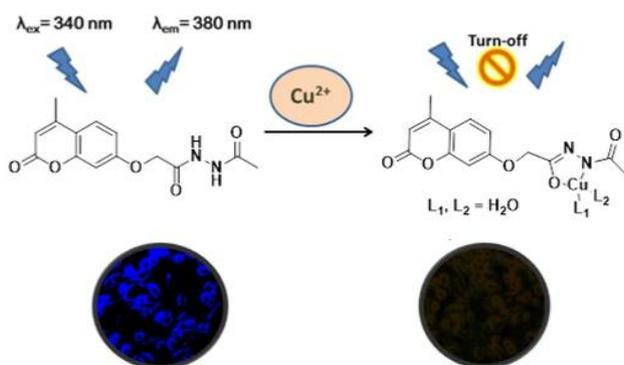
Fig. 17 presence of  $Cu^{2+}$  ion shown by fluorescence turn off.
