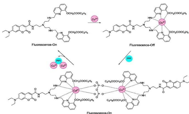
Fig 12 the mechanism showing fluorescence “ON-OFF” behaviour for  $Cu^{2+}$  and “OFF-ON” response for PPI.
