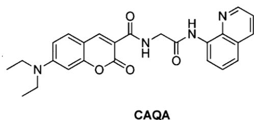
Fig. 19 structure of chemosensor CAQA for the detection of Cu<sup>2+</sup> ions.
