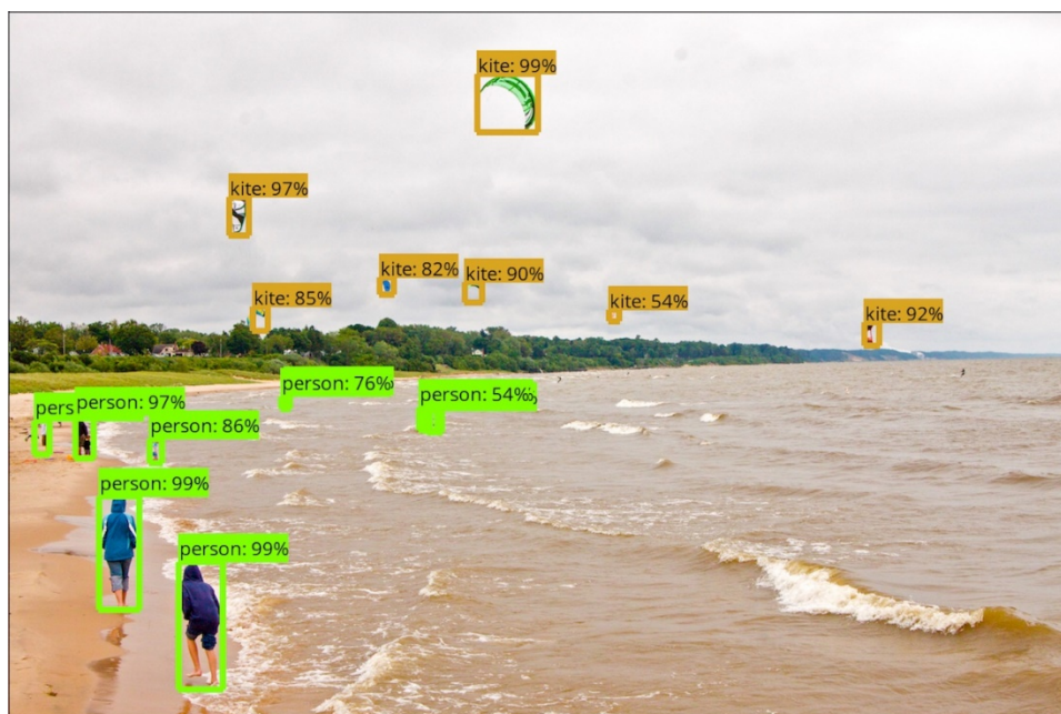
Figure 33: Example of object detection with confidence score [46]
