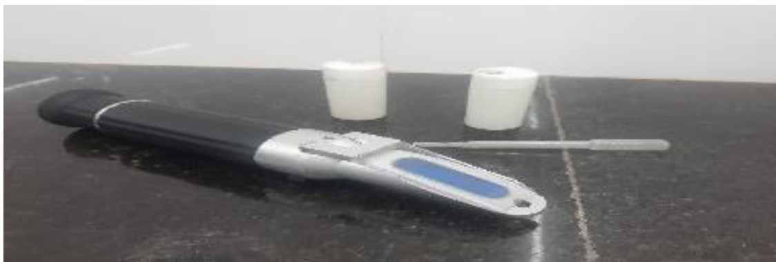
Figure 3.3: Salinity measured using MCP portable Handheld Refractometer
