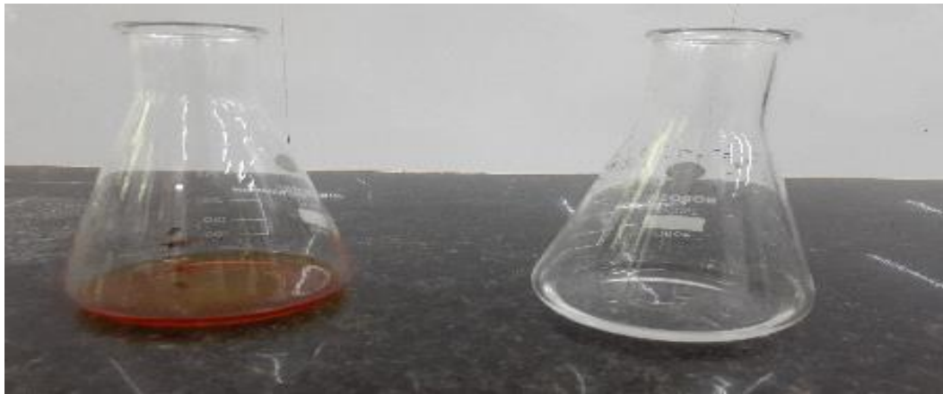
Figure 3.5: Water sample estimated for BOD colour change from initial colour (dark yellow) to end point (colourless)
