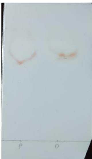
Fig 6. Thin layer chromatography: separation in Chloroform: methanol: ethylacetate
