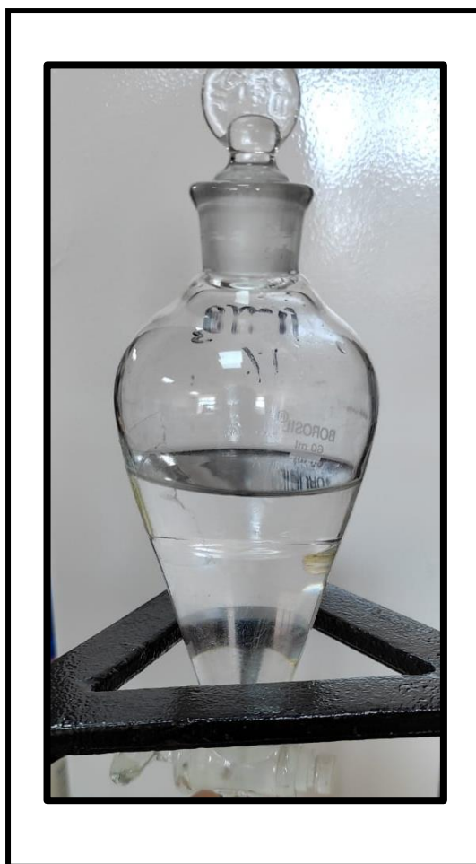
Figure 3.5: Partitioning crude extract in methanol and hexane using Borosil separating funnel
