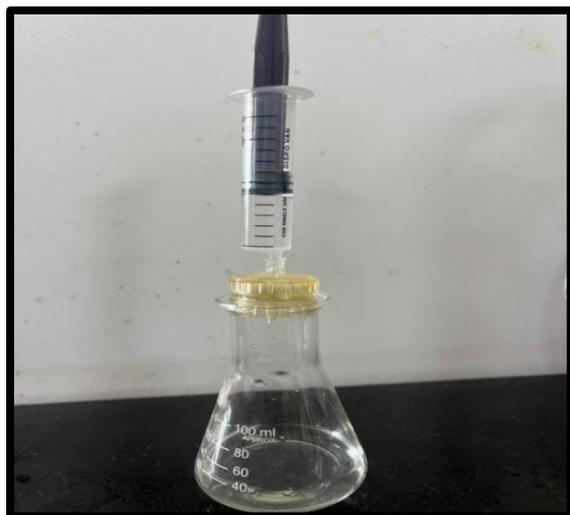
Fig 3.1: Filtered rainwater solution passed through 0.22 $\mu$ m filter using a 20 mL syringe.
