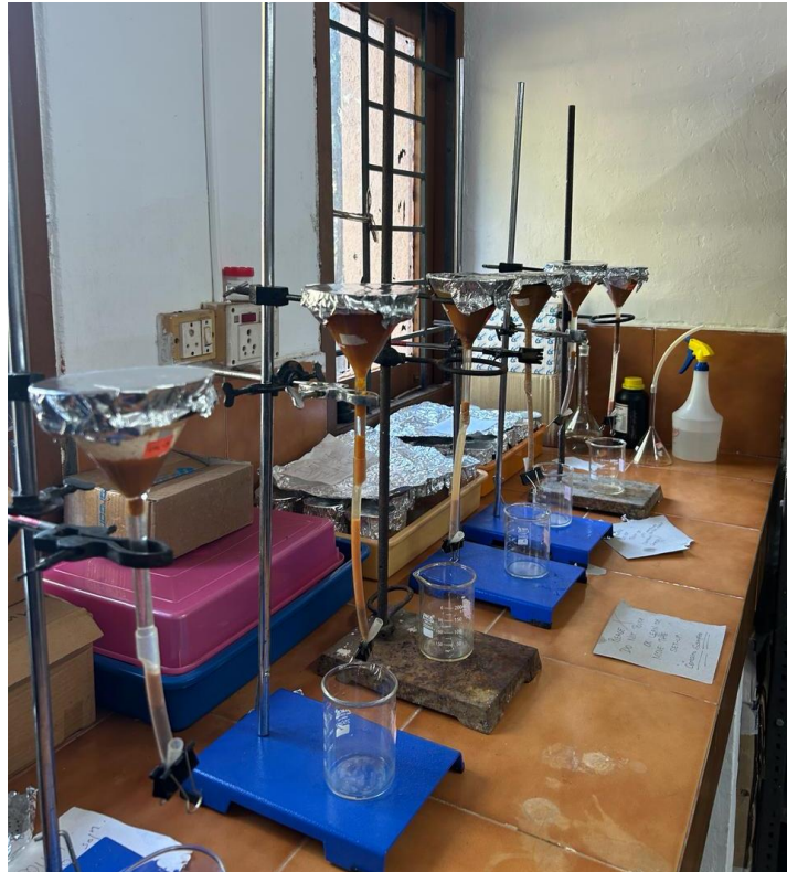
Fig 3.11: Gravity setup done for separating floating and settled solids
